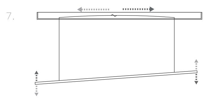
'Lines' can be leveled out by adjusting connecting wire left or right in the celing base.
